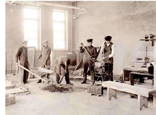
View of students mixing clay for placement in a small brick press, one of the hands-on activities of a course on practical brick-making offered at the Manitoba Agricultural College (Courtesy University of Manitoba Archives)
