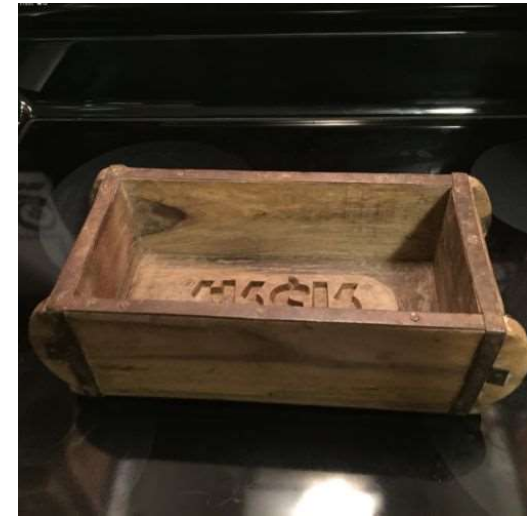
An old single-brick mould, the type used throughout the 19 th century for the production of bricks at small yards.
