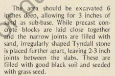
For heavily used areas, these wide grassed joints may not be satisfactory. A close fit and narrow joints between stones would then be preferable. This the low spots. If a more permanent can be achieved by cutting the stone on the construction site with appropriate stone cutting equipment to obtain the desired shape and size. The basic, random pattern is still maintained, although the sides of each stone consists of more or less straight lines.
