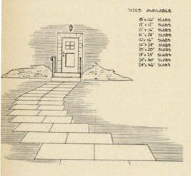
The spaces between the slabs are also filled with sand, gravel or wood chips. A wide variety of slab sizes will add interest to such an area.
