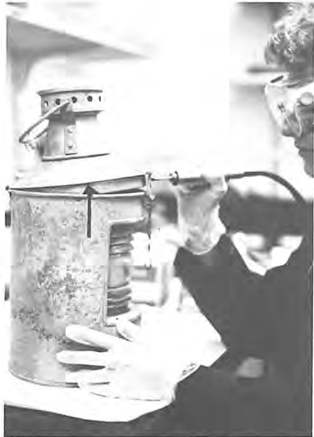
Surface cleaning metal with dental tool. Parks Canada
