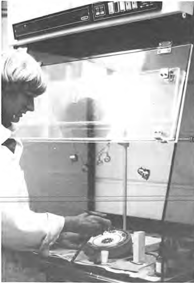
Inpainting ceramics with an air brush after mending. Parks Canada
