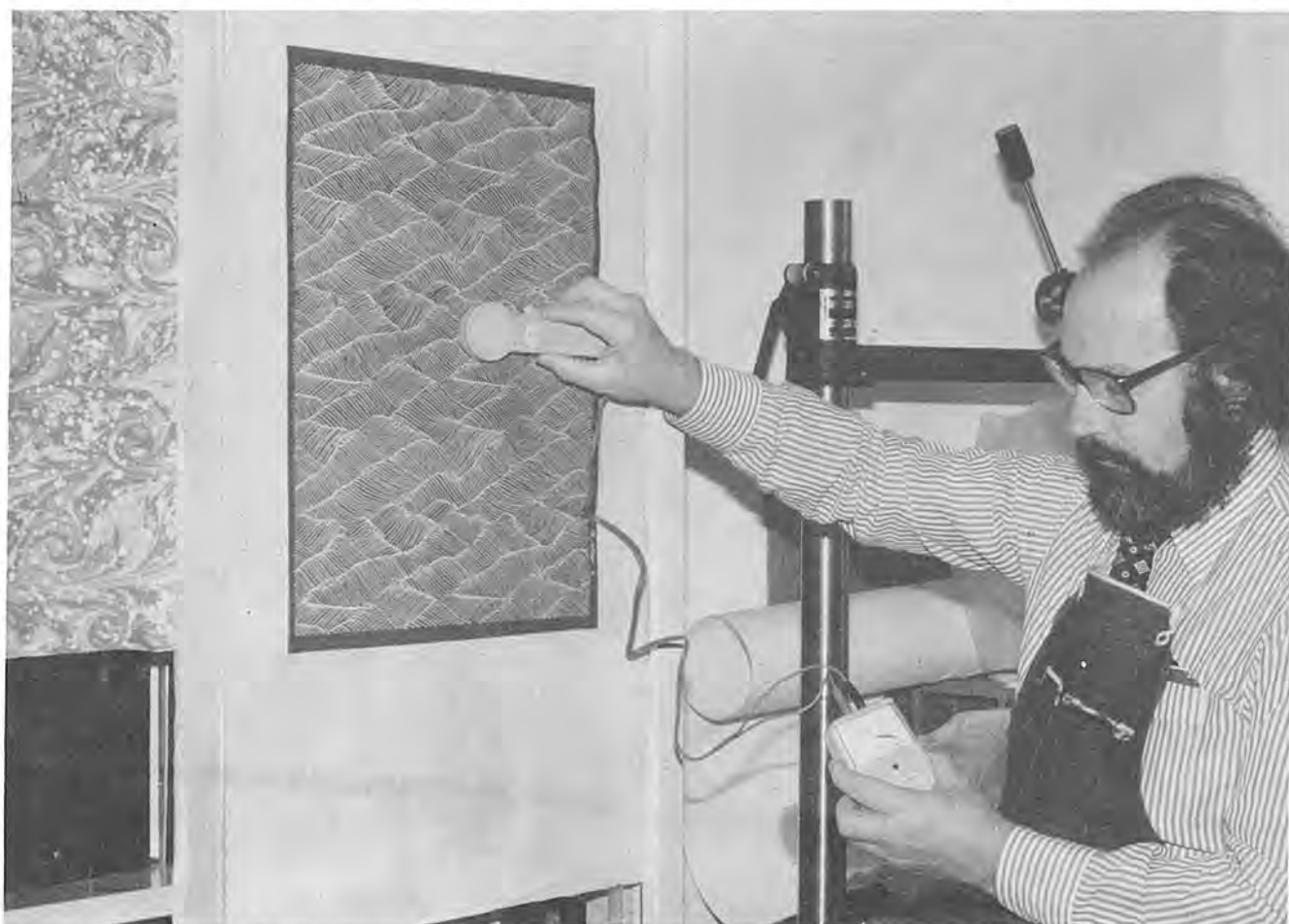
Measuring illumination falling on a work of art by means of a Panlux Electronic Luxmeter Provincial Archives of Manitoba
