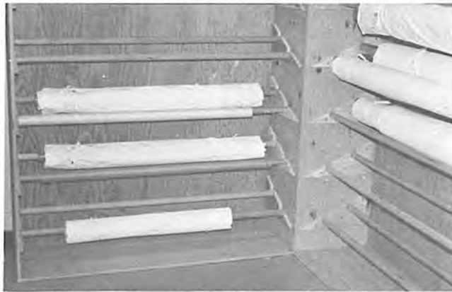
Two storage units were placed in a corner. By bolting them together at right angles, they reinforce each other
