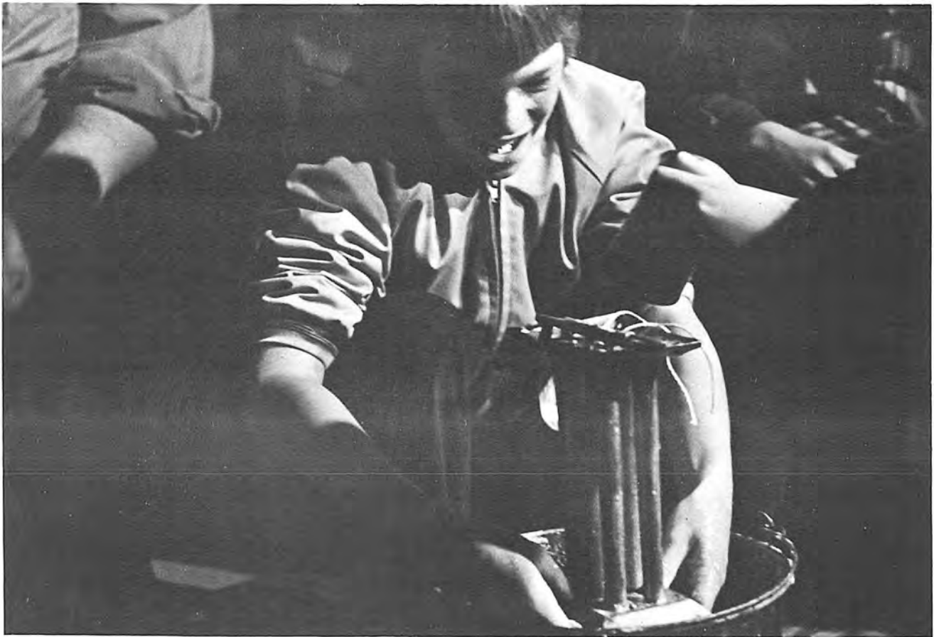
Teamwork helps to get the tallow into the mould
