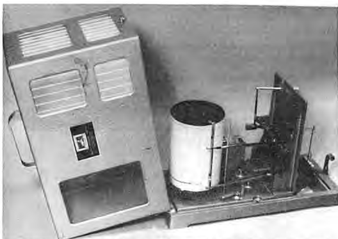
Recording thermohygrograph opened to show instrumentation. Sensors on right activate pens which record temperature and relative humidity on graph. W. Clearwater
