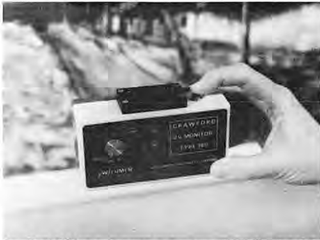
Crawford UV monitor measures proportion of ultraviolet radiation in the light falling on an object. W. Clearwater
