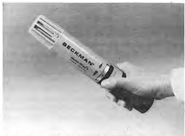
Beckman "Humichek". Sensors in head allow relative humidity to be read directly by rotating graduated dial with thumb. W. Clearwater
