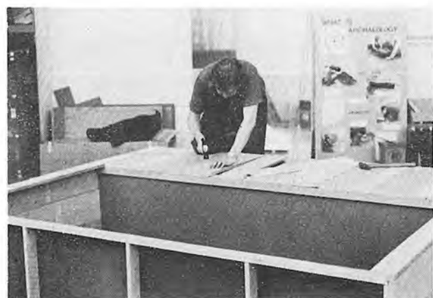
Figure 6 - Nailing on the front exterior
