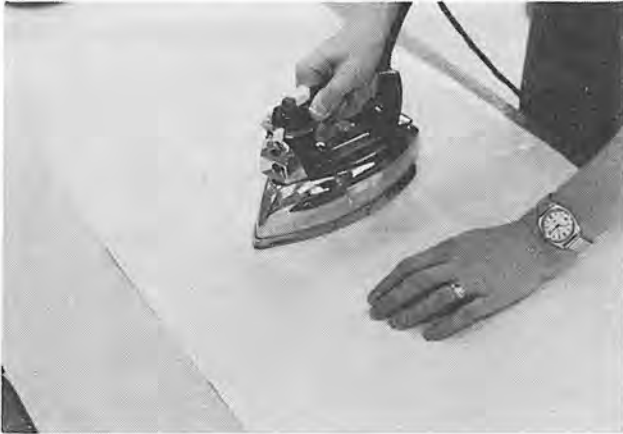
Dry mounting the work to the board
