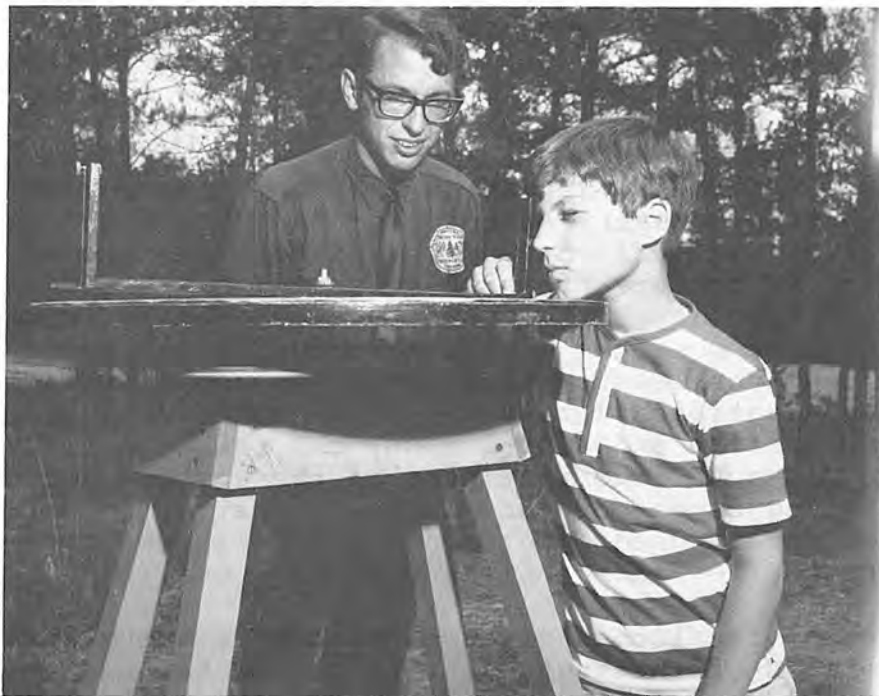
A young man demonstrating the use of an alidade which is used in locating forest fires
