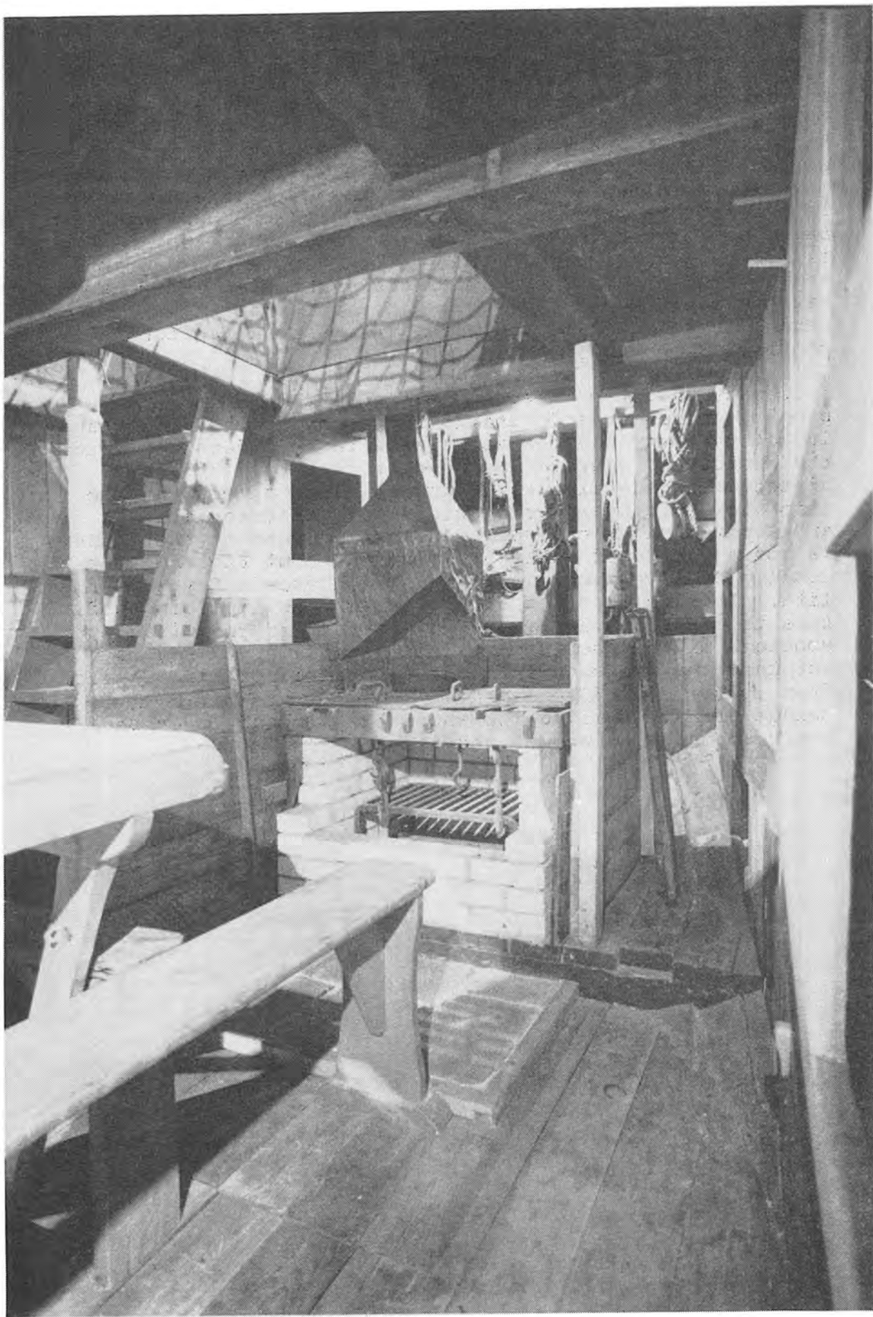
A stove and a smoke hood that constitutes the galley in the Nonsuch's hold
