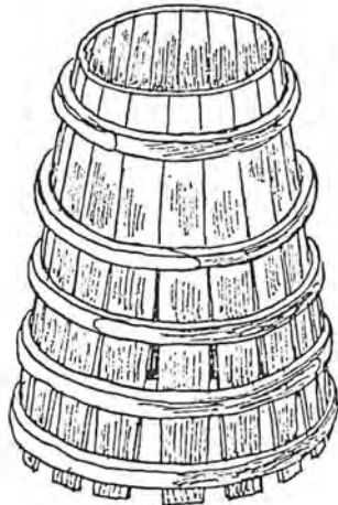
Raising staves in truss hoops
