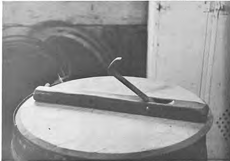
Flagging iron used to separate wooden staves when repairing wooden barrel
