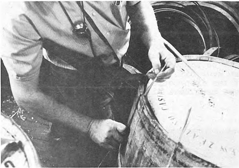
A flagging iron used to separate staves to insert bullrushes
