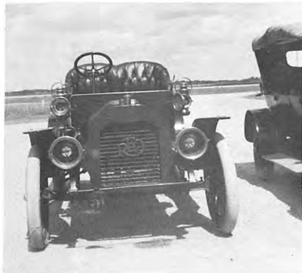
The Reo - a two cylinder, water cooled motor, with chain drive. It is in running condition
