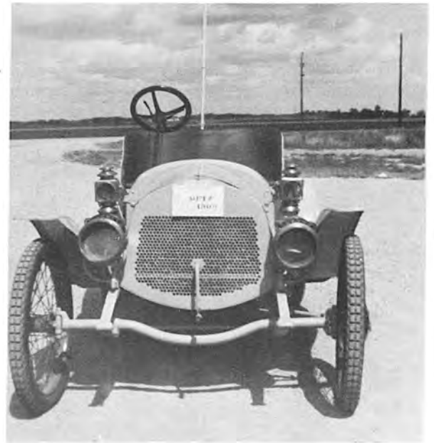
This small attractive car is a 1909 Metz, being a very rare auto, with not many of its kind still in existence. It has a two-cylinder, air-cooled motor, friction drive, and is still in running condition
