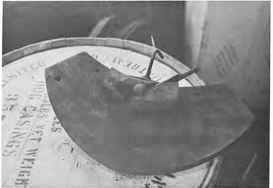
A chive used in shaping the top and inside of a barrel
