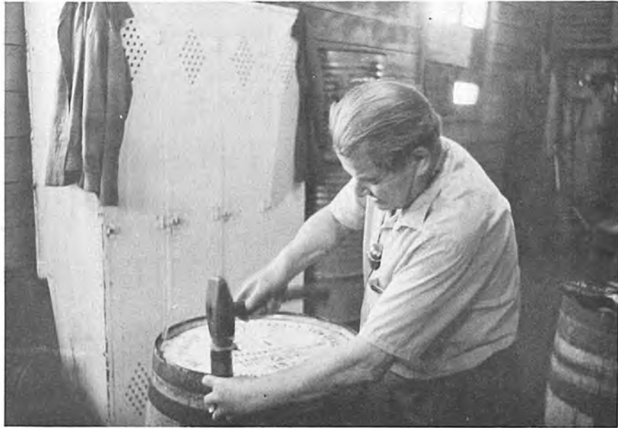
Replacing truss hoops after caulking with hammer and drive
